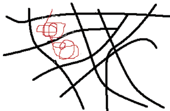
Figure 1. Mechanism for friction discussed here is illustrated for just two blobs for clarity. Dark lines represent polymers belonging to a polymer brush. The red lines represent a polymer that has penetrated into the brush represented by the dark lines. The mesh spacing in which these blobs reside are of size \xi , which is actually a correlation length, rather than a static mesh spacing. 10 Its size is exaggerated here. In reality, \xi is only a factor 2 larger than the mean intermonomer spacing within an interpenetrating blob.
